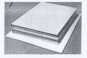
4. AFTER SETTING, REMOVE THE WEIGHT AND SIMPLY PEEL OFF THE PLASTI-CARD, EXTRACT THE CASTING IN THE NORMAL WAY.
